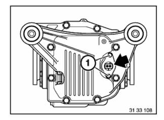
Unfasten screws (1) and remove speedometer-display sensor.
