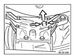
Disconnect plug-in connection at rear axle.
